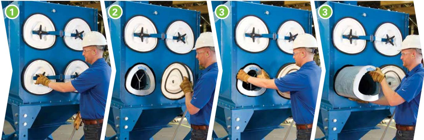
**1** Loosen cover with 4-lobe knob. Knob has center lug enabling power tool operation.
