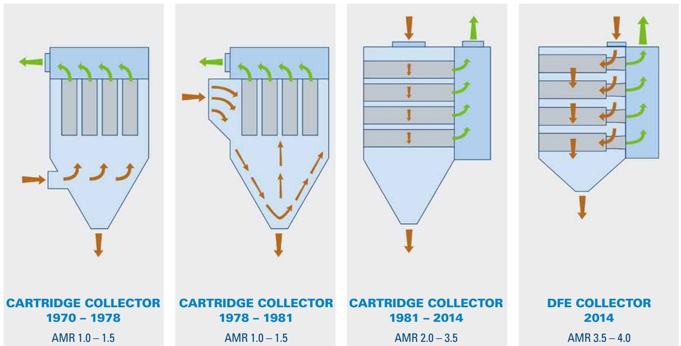
The graphic above shows an example of the Air-to-Media ratios for a typical weld fume application. The DFE features higher AMRs, smaller footprint, fewer filters, superior performance, and lowest cost of ownership!
